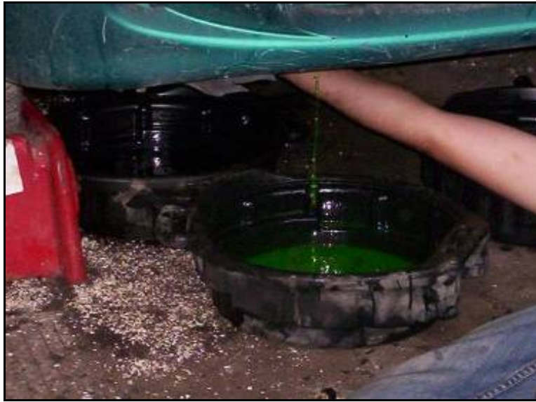
Figure 11: Using Drip Pans to Catch Draining Fluids
