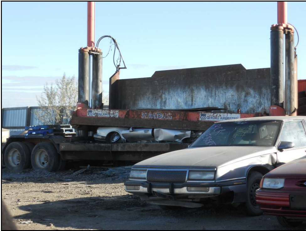
Figure 5: Vehicle Crusher in Operation
