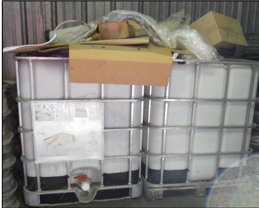
Figure 4: Example of Plastic Totes Used for Collection of Vehicle Fluids - Not Used for Gasoline
