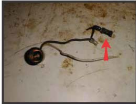
Figure 18: Chest Freezer Light with an Inline Mercury Switch (Glass Ampule)
