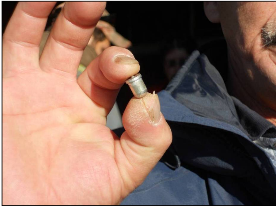
Figure 16: Mercury Pellet removed from Vehicle Convenience Light
