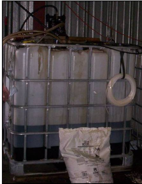
Figure 13: Example of Plastic Container Used for Storage of Waste Oils
