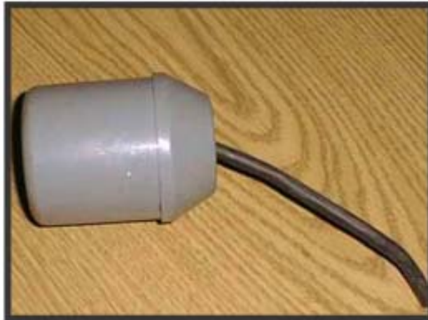
Figure 21: Sump Pump Float Containing Mercury
