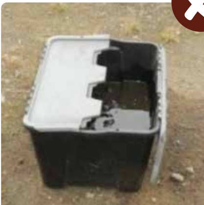
IMPROPER storage of waste oil
