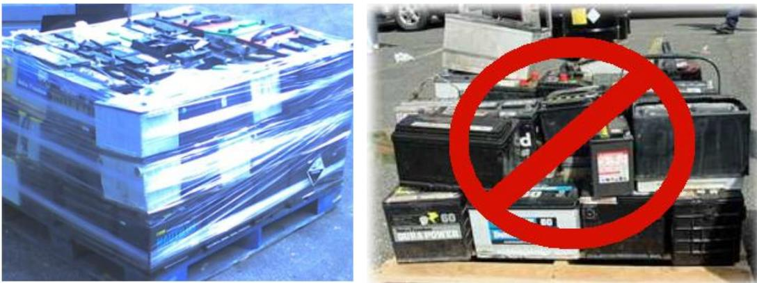
Figure 2 – The Proper and Improper Storage of Lead-Acid Batteries
